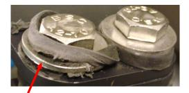
Figure 4: Sharp Edge of the Washer Against the Shock Isolator
